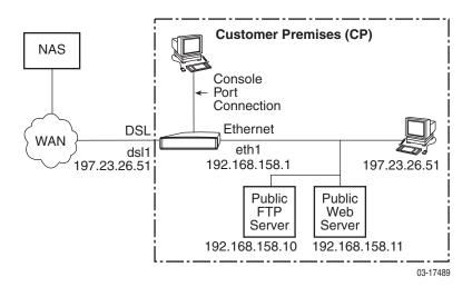
In this example, the 6351 router shares its public IP address with another device. NAPT is configured to support public FTP and web servers connected directly to the router's LAN interface. These servers share the same public IP address as the passthrough device and are accessible to remote users via the configured static NAPT mappings.
